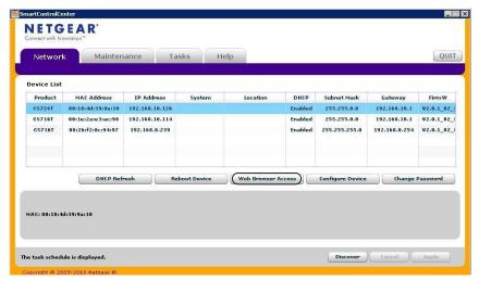
The Smart Control Center Utility finds the switch and displays its MAC Address, IP Address, and model number. If you cannot configure your switch, verify that the cable connections are secure, that the IP address configuration of the PC is in the same subnet as the switch, and click the Discover button.
